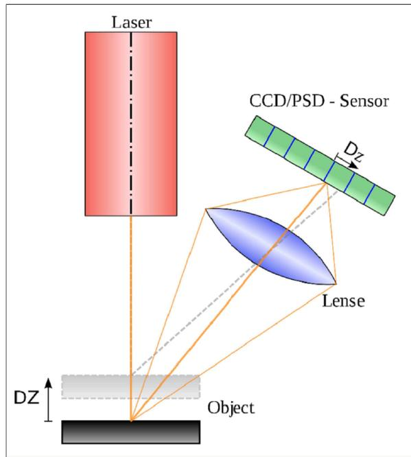
Figure 1. Principle of laser triangulation
