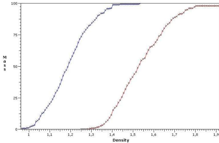
**Figure 11. Washability curves with the summed up mass over the density**
