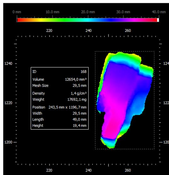
**Figure 7. Analyzed coal particle with calculated parameters**
