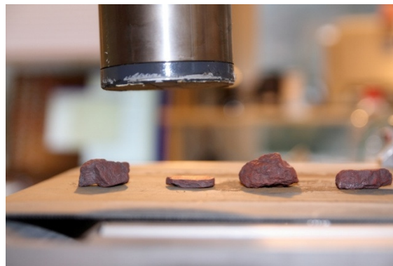
Figure 3. X ray measuring path mounted on a small conveyor
